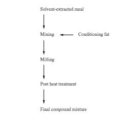
Apparatus for Treating Solvent-Extracted Plant R sidu
